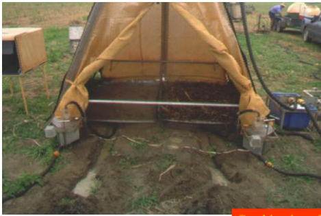
Combination of Compaction and unstable aggregates
